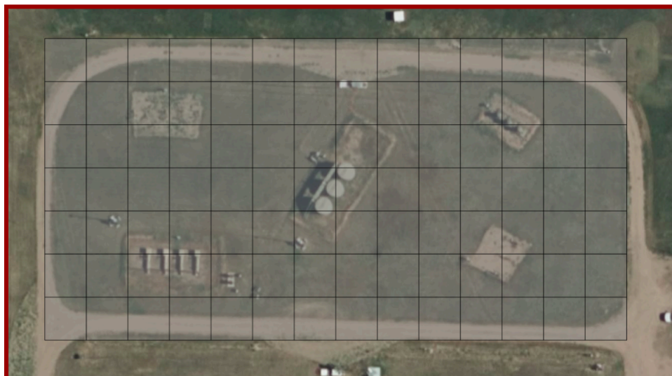
Figure 1: METEC ADED site from 2024 where single-blind testing was performed. The site is 140 meters across in the east-west direction and 70 meters across in the north-south direction. Each square in the grid is 10mx10m
