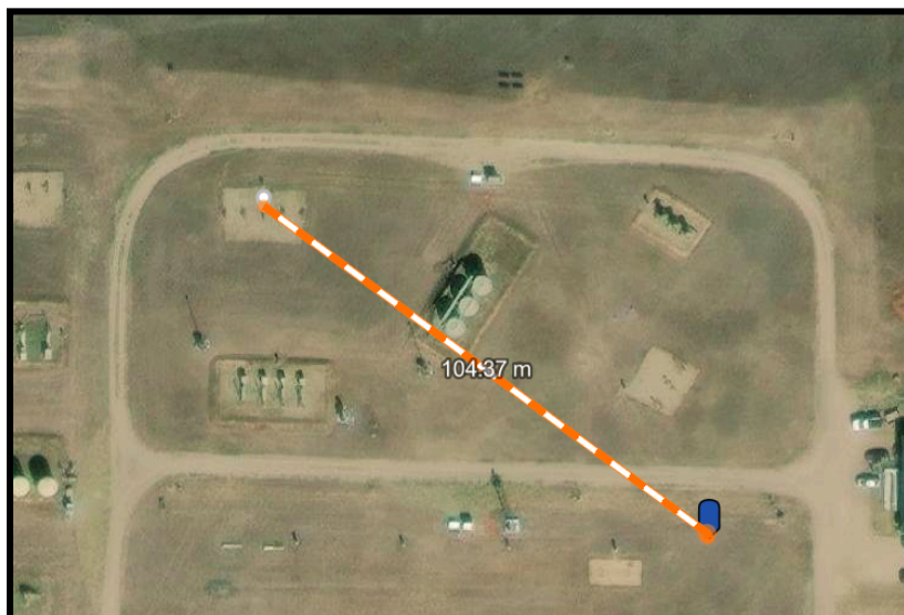
Figure 8: Experiment 2 detection results from a 0.63 kg/hr leak from 4W-3 wellhead detected by MT: 5 device at a distance of 105m .
