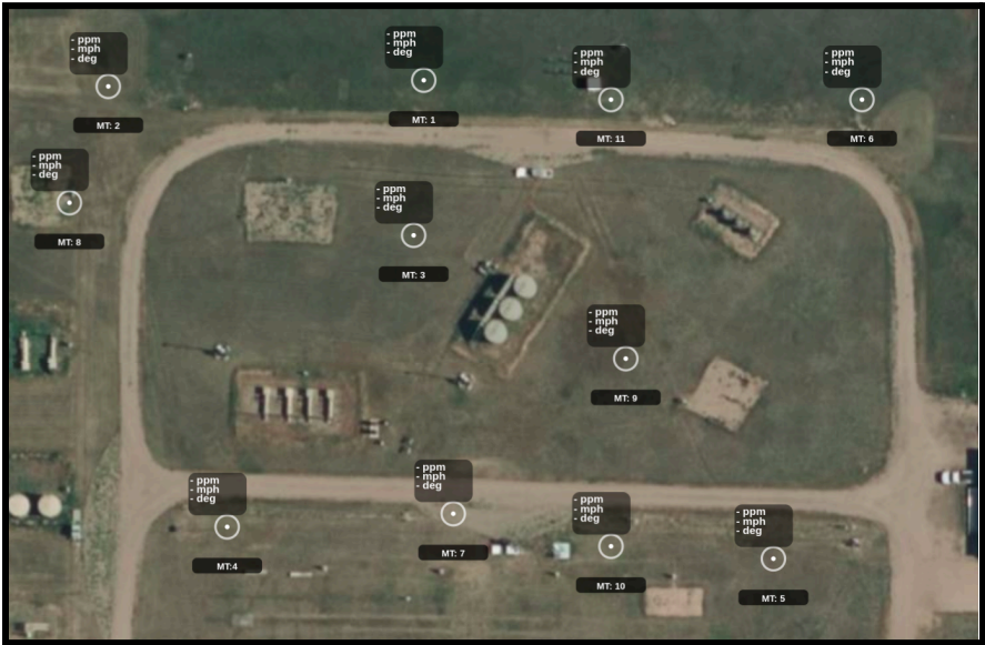
Figure 3: Earthview IoT device placement at the METEC ADED Facility in 2024 testing. Devices are labeled “MT 1-12”.
