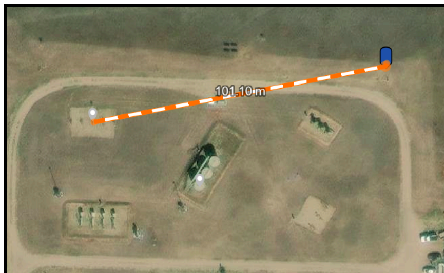
Figure 5: Experiment 1 detection results from a 1.5 kg/hr leak from 4W-3 wellhead detected by MT: 6 device at a distance of 101m .
